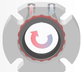
Tangential ports and pumping ring (red) provide effective, forced circulation
