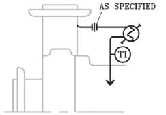
**Description:** Plan 21 is recirculation from pump discharge through an 1/8" minimum flow control orifice (when necessary), and seal flush cooler, then into the seal chamber.
