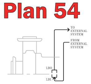
**Description:** Plan 54 is an external system supplying clean BARRIER fluid to an Arrangement 3 dual seal at greater pressure than the process pressure being sealed. Pressure and circulation are provided for by an external pump or pressure system.
