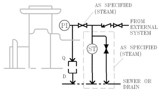
**Description:** Plan 62 is an external source supplying quench (nitrogen, water, steam, etc.) on the atmosphere side of the seal. Typically used with a throttle bushing or auxiliary sealing device for containment.
